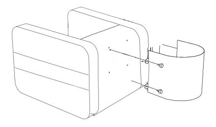
STEP 2:-With the 4 bolts provided, screw the steel pedestal into the back of the chair. (Note: If this is already installed, go straight to Step 3)
