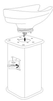
STEP 3:-Carefully place the basin bowl and tilt through the 4 holes in pedestal.
