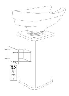
STEP 2:-Open the rear panel of the pedestal unit by removing the 4 screws.
